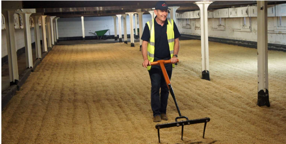
Lower malting floor, after water is drained out. Note the raised cistern. The maltster would turn grain to encourage growth. Louvered window panes would provide air circulation.
